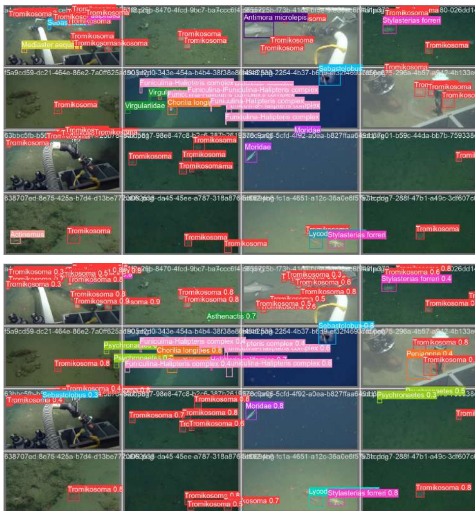
Figure 5.4: (a) The ground labels for object detection. (b) The predicted labels by yolov9 object detection model.
