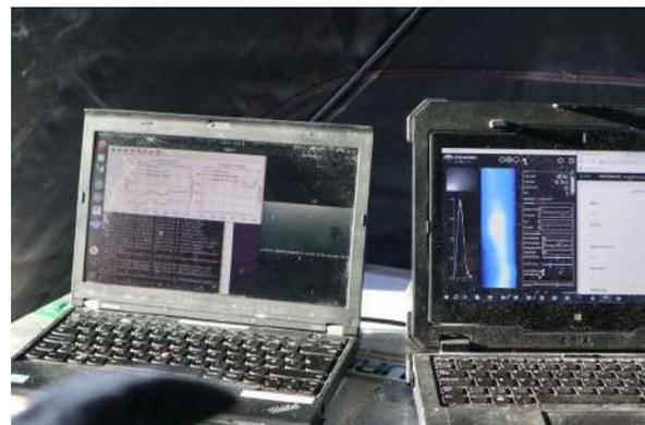
Figure 4.5.b: Topside units of DBE setup. The laptop on the left shows the DVL script and RGB camera feed of the robot. This laptop is also used to control the DBE. The *Immersion* software is running on the right laptop, showing the live hyperspectral data, visualized as RGB imagery, the UHI's RGB camera feed, and the optical signature of the hyperspectral data.
