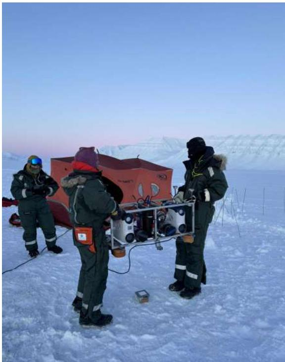
Figure 4.8: Reflected radiance measurements; the UHI is pointed down, towards the Spectralon reference plate.
