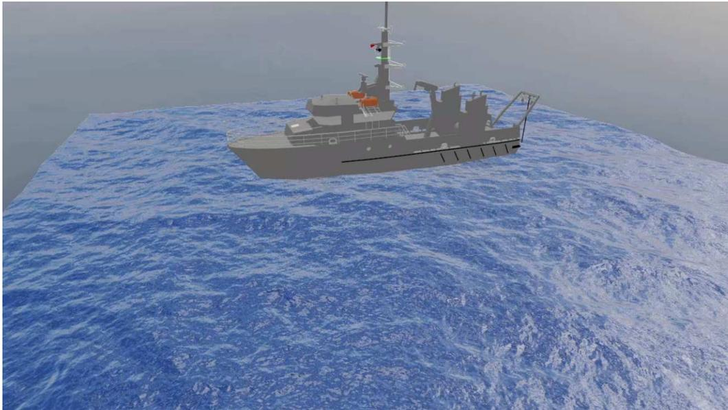
Figure 5.3: Implementation of wave sim plugin in Gazebo sim
